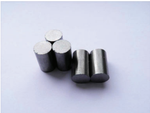
Figure 3. Sintered NiAl/Al 2 O 3 specimens.
